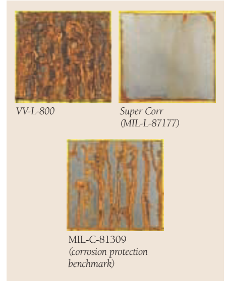
FIGURE 2: A second round of tests determined that the lubricating and corrosion protection properties of Super Corr were superior to the product being used by the P-3 squadron at NADEP Jacksonville.
